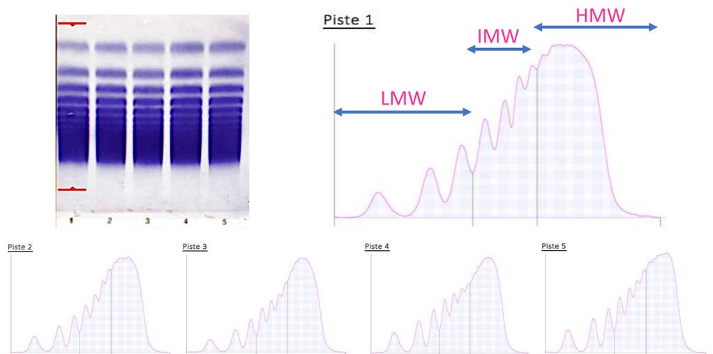
**Figure 4.** Inter-sample contamination
